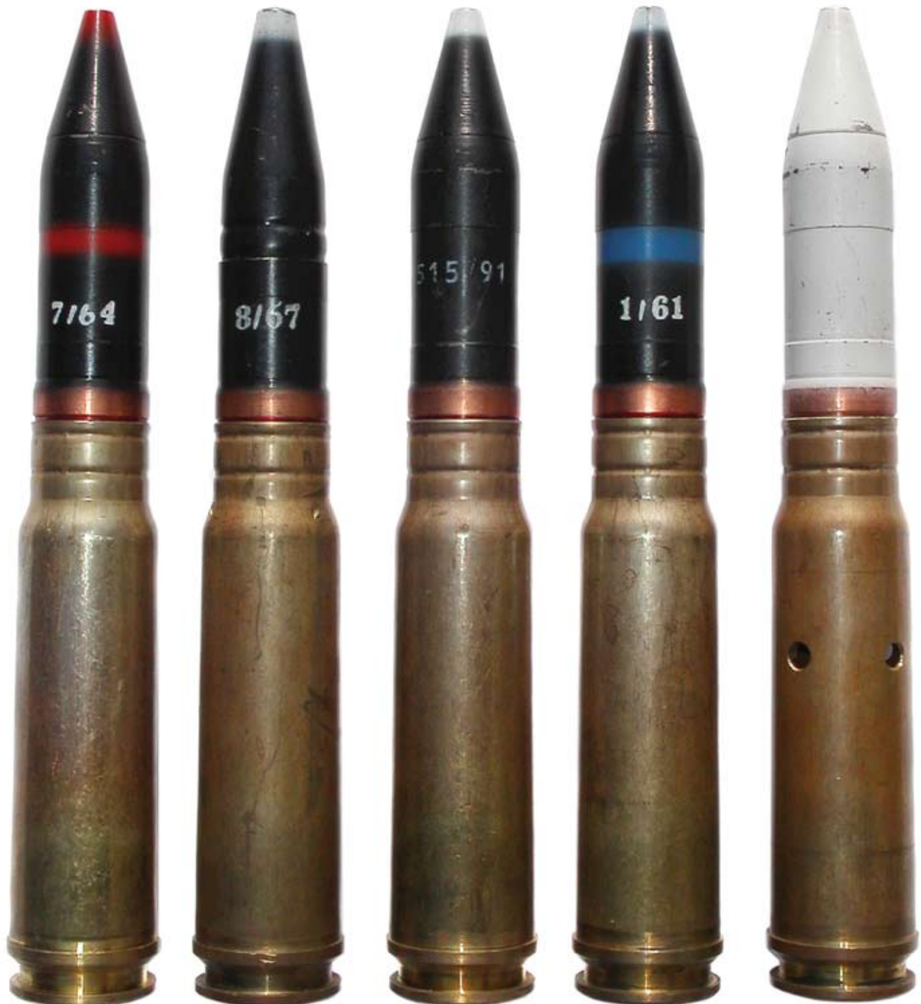
Czechoslovakian NR-30 cartridges from left to right: OFZ, LP-3, LP, reference and drill round. While the other rounds were made during the 1960's, the LP target practice projectile was made in 1991. The reference cartridge consists of a standard LP round and is identified by a blue band.
